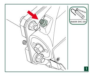
7.3.6 Lubricate the S-cam bearing
