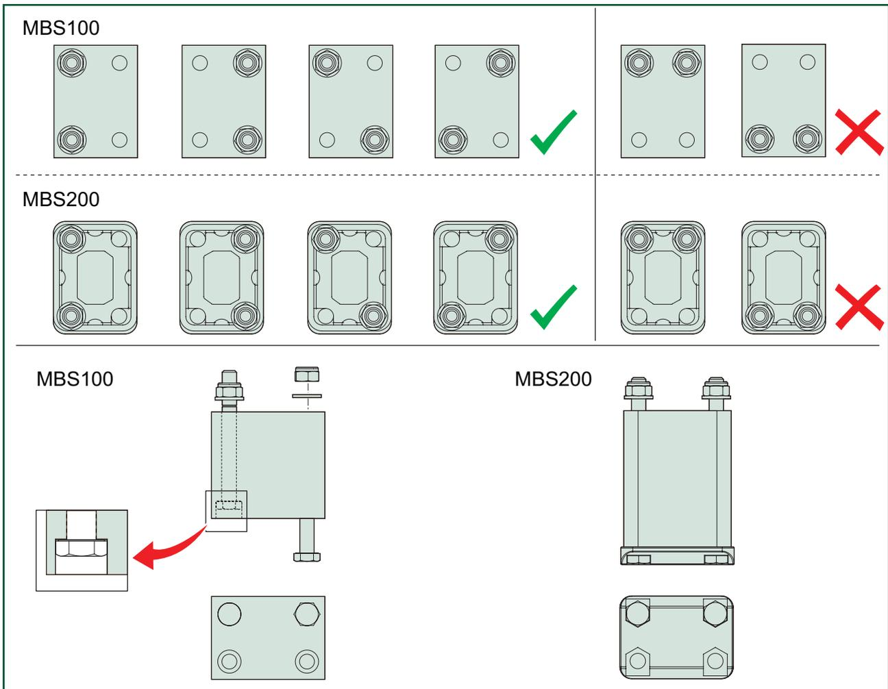
**i** The long side of the bump stop must be positioned parallel to the trailer flat.
