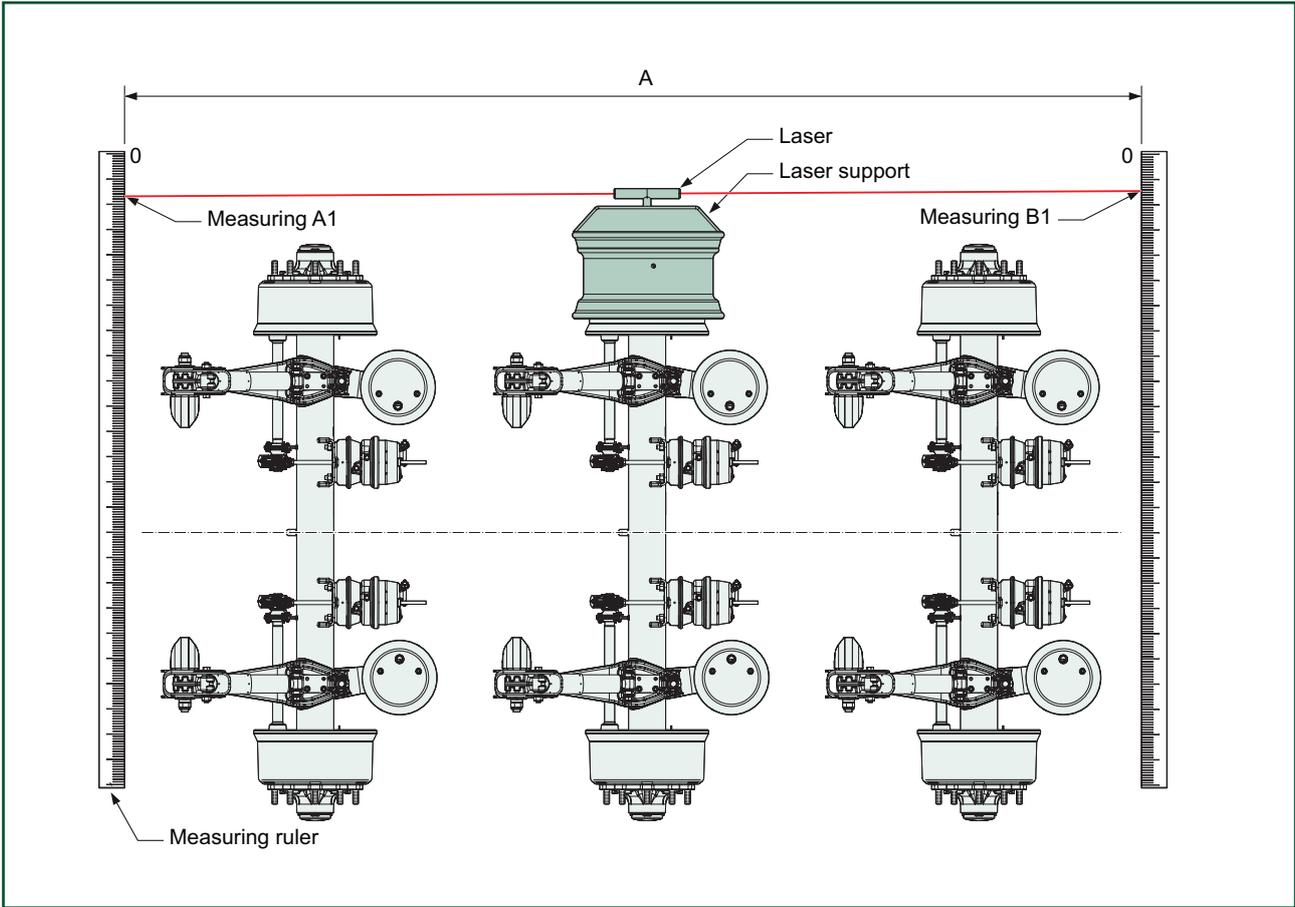
**i** The figure shows the drum brake axle. Positioning the tool for the disk brake is the same. The tolerances as given in section 5.2 remains the same.
