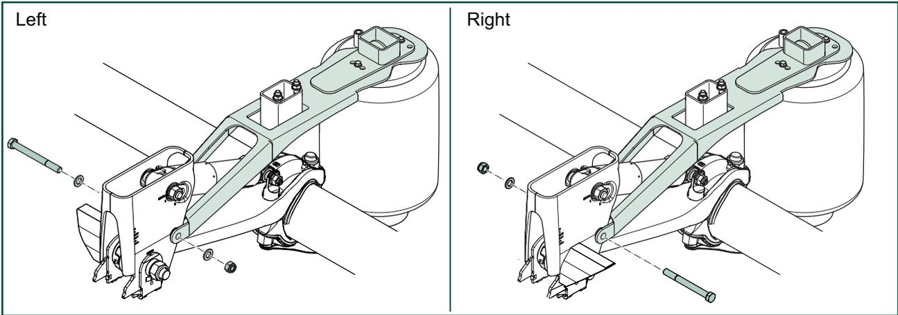
**i** To facilitate replacement of the splitter, always fit the mounting bolt on the inside.
