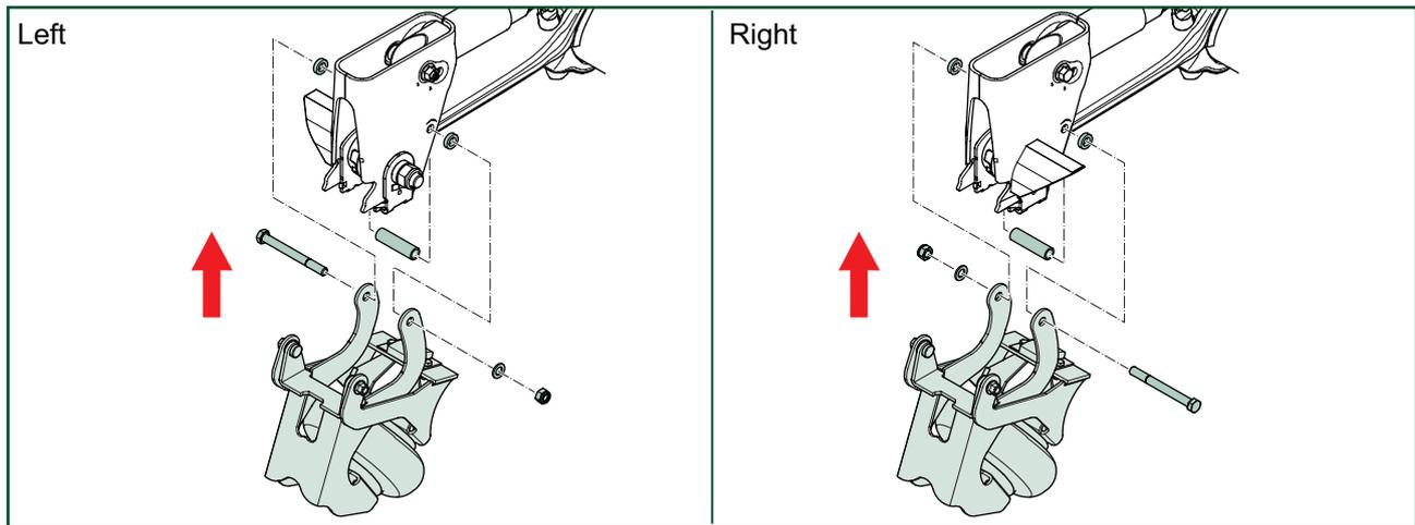
**i** To facilitate replacement of the axle lift, always fit the mounting bolt on the inside.
