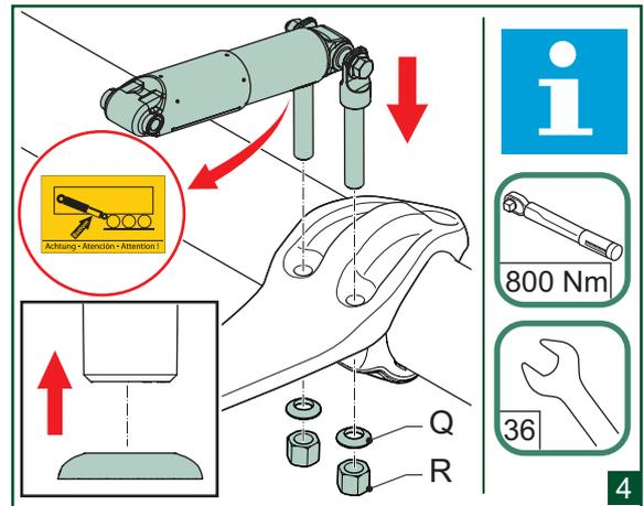
**i** For the tightening torque of the axle clamp (front), see section 6.1. Always tighten nuts (R) before tightening nuts (U)!
