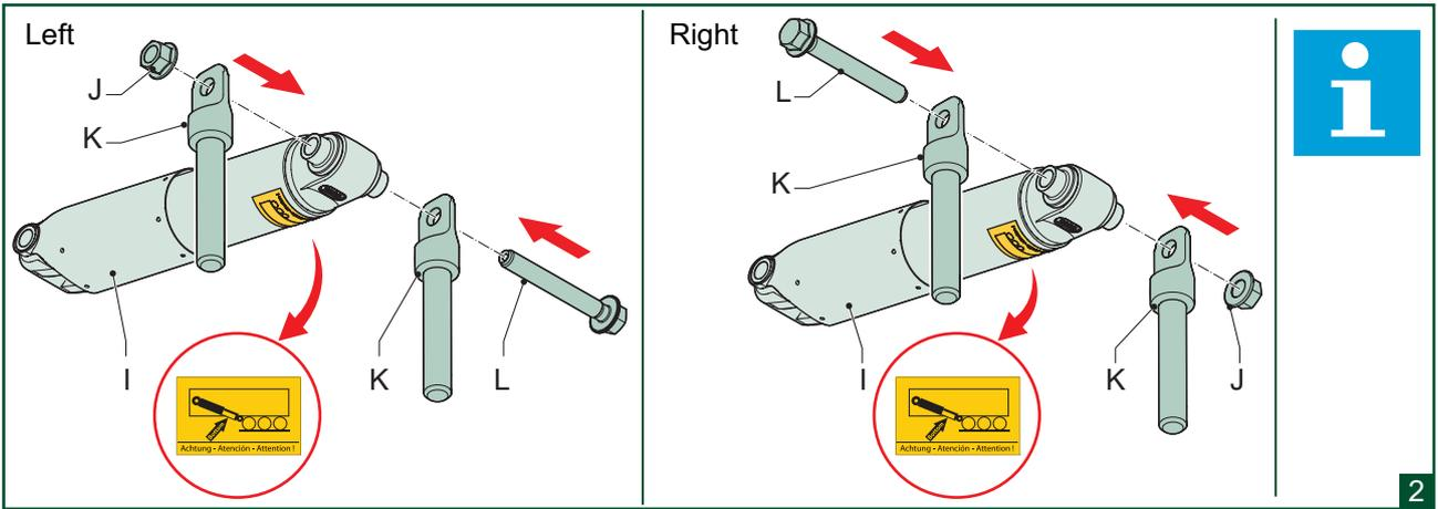
**i** To facilitate replacement of the shock absorber, always fit the lower shock absorber bolt from the inside. So per axle, left and right differ!
