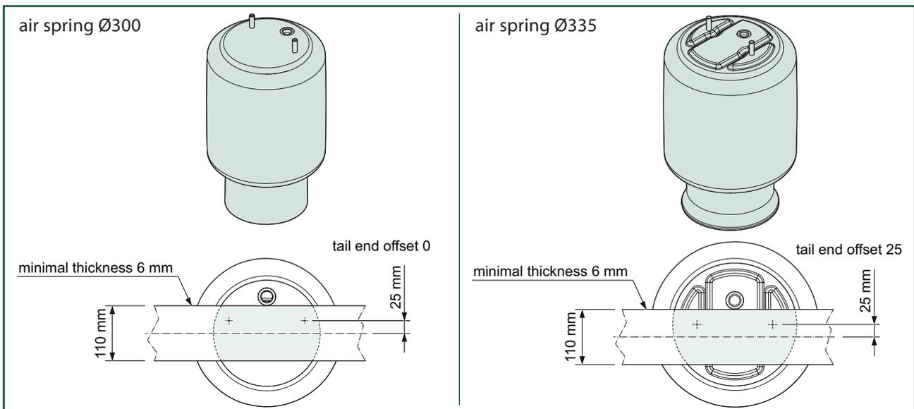
**\*If chassis is less than 110 mm a support plate min. 110 mm has to be added!**
