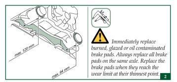
Check the condition of the brake disk
