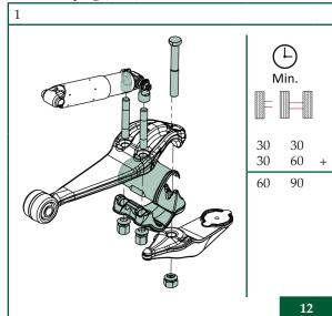
Pivot bolt connection and wear plate
