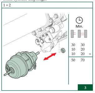
Brake anchor plate and brake caliper
